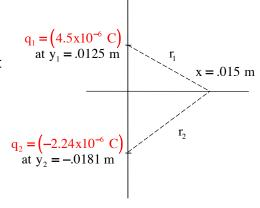
$$V_{\text{origin}} = k \frac{q_1}{|r_1|} + k \frac{q_1}{|r_2|}$$
